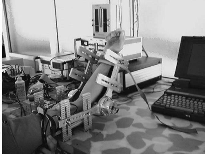
Figure 6.12: The isometric brace used to keep the elbow angle constant at 120 degrees during the acquisition of surface EMG signals. Torque sensors are located at the joint of the rigidly connected parts of isometric brace (source: LISiN, Politecnico di Torino, Italy).
